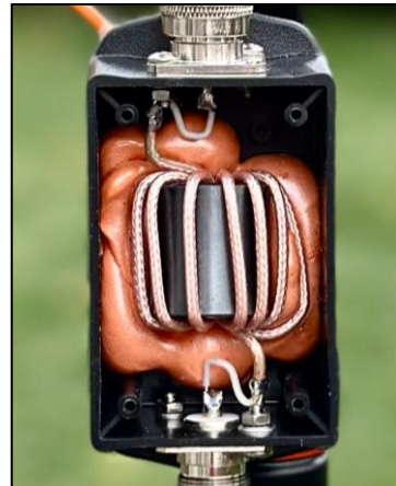
MC-1-500-50 Ferrite Bead Mix 31 0.687" O.D. x 0.375" I.D. x 1.125" Height
