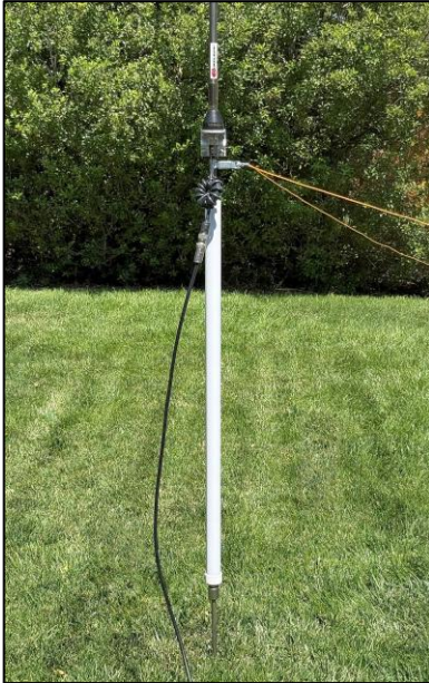
PERformer Quarterwave with 2 Elevated Radials
