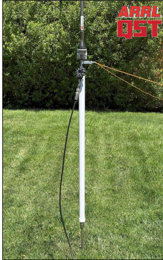
PERformer shown with a 40" furniture-grade PVC tube on a stainless-steel ground spike.
