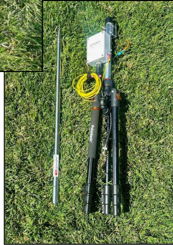
The LDG™ 4:1 unun or the TennTennas™ 49:1 with RF choke are already mounted to the tripod for fast and easy deployment.
