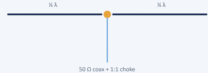
Half wave, center fed, current maximum in the middle
